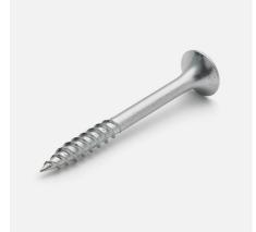
**Function:** Straight tip with double thread grooves that grip immediately, penetrate the steel plate very quickly and sink into the drywall board without damaging the cardboard layer. Suitable for drywall installation where the inner board is made of chipboard or plywood.
