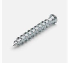
**Function:** Sharp tip and threads adapted for anchoring in wood or drywall to drywall. The threads immediately grip and tighten the screw to the drywall without damaging the cardboard layer. Suitable for installation of second layer of drywall directly onto the first drywall board. Second layer of drywall is adhered prior to assembly.
