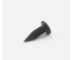
**Function:** Round washer head screw with low head and our patented TRUSTGO design. The screw has a straight tip and double thread groove that grip immediately and goes through the steel plate without forming any steel chips. The design of the double thread groove provides a stable assembly with high pull-out value.
