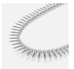
Function: Drill tip with single thread steel grooves, drills very quickly in steel thicknesses up to 2 mm, and sinks into the drywall without damaging the cardboard layer.
