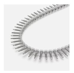
**Function:** Drill tip with single thread steel grooves, drills very quickly in steel thicknesses up to 2 mm. The screw meets the requirements in AMA Hus 24 KBC.3111 for the installation of external wind protection plates. Suitable for installing external drywall boards.
