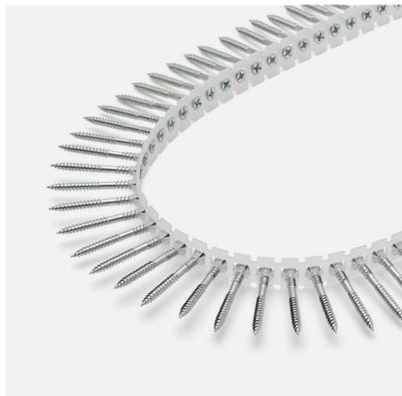
**Function:** Sharp tip with double thread grooves that grip immediately and penetrate the steel plate very quickly. The reversing threads underneath the head allows the screw to sink into the drywall board without any problems.
