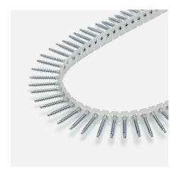
Function: Drill tip and threads adapted for anchoring to wood and steel up to 2 mm. The design of the head allows the screw to sink into the drywall board without any problems. Suitable for mounting extremely hard drywall board.
