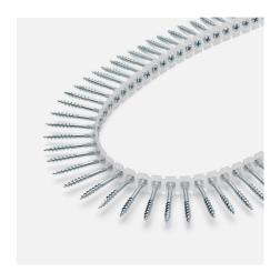
Function: Sharp tip and threads adapted for anchoring in wood. The threads grip immediately and tighten the screw to the chipboard, while the grooves underneath the head sink the screw. The screw also has a cutting drill tip to prevent cracks forming in the wood. Suitable for assembly of chipboard, OSB, Plywood and other wood-based boards.
