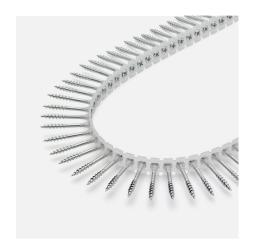
Function: Sharp tip and threads adapted for anchoring in wood. The threads grip immediately and tighten the screw to the chipboard, while the grooves underneath the head sink the screw. Suitable for assembly of chipboard, OSB, Plywood and other wood-based boards.
