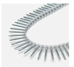
**Function:** Drill tip and threads adapted for anchoring to steel up to 2 mm. The wings mill out the hole in the timber. When the drill tip passes through the steel the wings break off. The grooves under the head sink the screw. Suitable for assembly of chipboard, OSB, Plywood and other wood-based boards.
