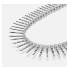
**Function:** Drill tip and threads adapted for anchoring to steel up to 2 mm. The wings mill out the hole in the timber. When the drill tip passes through the steel the wings break off. The grooves under the head sink the screw. Suitable for assembly of chipboard, OSB, Plywood and other wood-based boards.
