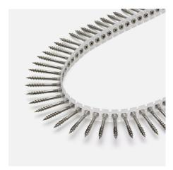
Function: Sharp tip and threads adapted for anchoring in wood. The threads grip immediately and tighten the screw to the decking, while the grooves underneath the head sink the screw. The screw also has a cutting drill tip to prevent cracks forming in the wood. Suitable for installation of decking, balconies, fences etc.
