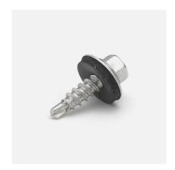
**Function:** Drill tip for aluminium sheet up to 2 x 1.25 mm. Sheet metal thread for overlap function. Hexagon head with flange for safe tightening. Sealing washer for secure seal.
