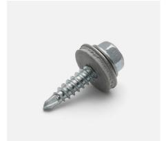
**Function:** Drill tip for sheet metal up to 2 x 1.25 mm. Sheet metal thread for overlap function. Hexagon head with flange for safe tightening. Sealing washer for secure seal.
