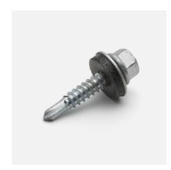
**Function:** Drill tip with diameter adapted to suit sheet metal, drills in beams from 1.3 mm up to 4.0mm. Steel thread provides solid anchoring in the beam. Hexagon head with flange for safe tightening. Sealing washer for secure seal.
