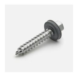
Function: Wood thread type A provides solid anchoring in timber. Hexagon head with flange for safe tightening. Sealing washer for secure seal. Recommended for use in pre-drilled sheet metal to wood.
