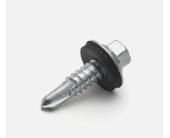
**Function:** Drill tip with diameter adapted to suit sheet metal, drills in beams up to 6.4 mm. Hexagon head with flange for safe tightening. Sealing washer for secure seal.
