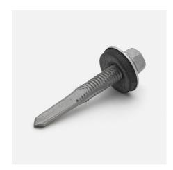
Function: Drill tip with diameter adapted to suit sheet metal, drills in beams from 4.0 mm up to 12.5 mm. Hexagon head with flange for safe tightening. Sealing washer for secure seal.
