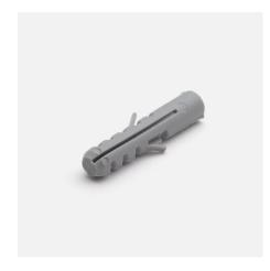
**Function:** Solid plug with good temperature and ageing properties. The plug design prevents any rotation when installing and allows for targeted anchoring. The plug can be used with most building materials, but is best suited in solid materials such as concrete, stone and solid tile.
