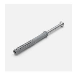
**Function:** Solid nylon plug with good temperature and ageing properties. The façade plug has a four-sided anchoring section and is designed to be used with most building materials such as concrete, lightweight concrete, hollow block etc.
