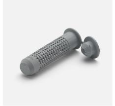
**Function:** The perforation sleeve is used together with the chemical anchor for attachment to hollow block. The sleeve causes the chemical anchor to form a body around the part to be fixed to the hole.
